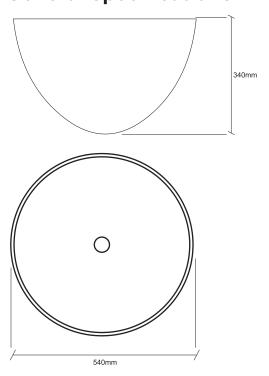
The slimline range of wallmount basins are manufactured using Paradyne's sygnite quartz composite materials. Solid moulded basins, these basins are available in a variety of shapes, sizes and finishes, catering to the overall design of any bathroom.
